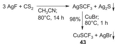
Scheme A.16 Preparation of the trifluoromethylthio copper(I) reagent [23].
