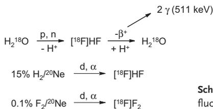
**Scheme 4.38** Methods for generation of  $^{18}\text{F}$ -labeled fluoride or hydrogen fluoride [83].
