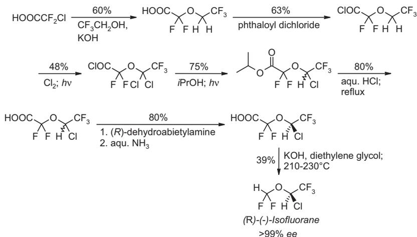
**Scheme 4.43** Synthesis of enantiomerically pure (R)-(-)-isoflurane [100].
