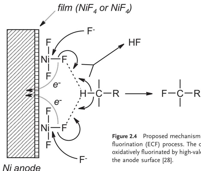
**Figure 2.4** Proposed mechanism of the electrochemical fluorination (ECF) process. The organic substrate is oxidatively fluorinated by high-valence nickel fluorides at the anode surface [28].
