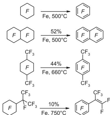
**Scheme 2.27** Industrial-scale methods for reductive defluorination–aromatization of perfluorocycloaliphatic precursors, which again are accessible by the cobalt trifluoride process [74].
