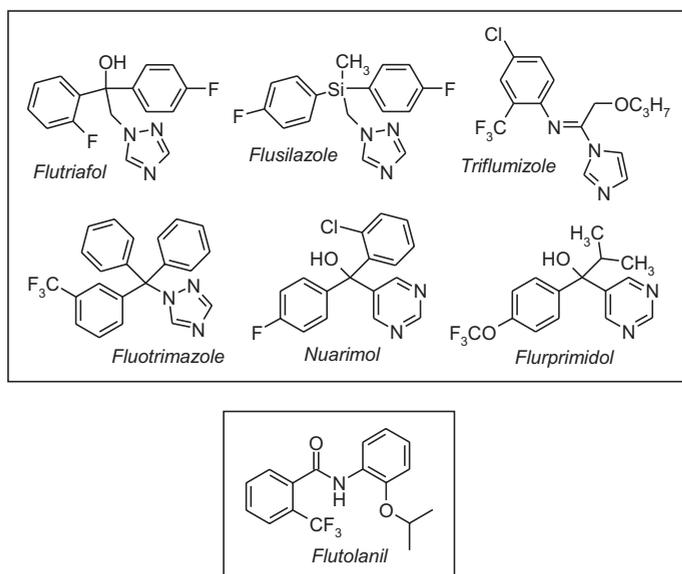
**Scheme 4.46** Different examples of fluorinated fungicides: (top) sterol biosynthesis inhibitors and (bottom) a benzamide-based compound [15–22].
