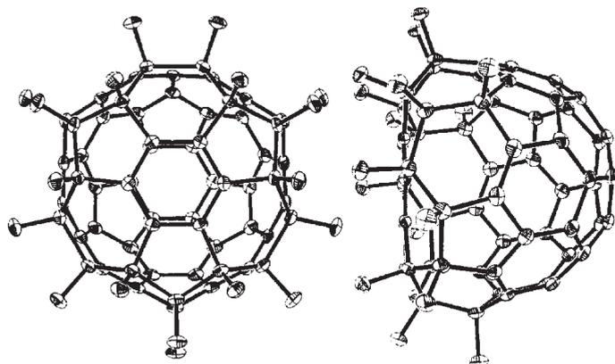
**Figure 2.3** X-ray structure of  $C_{60}F_{18}$  obtained by selective fluorination of  $C_{60}$  with  $K_2PtF_6$  without solvent at 230–330°C [15].
