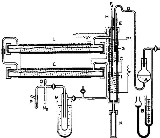
Figure 2.1 Fluorination apparatus used by Bigelow and Fukuhara for perfluorination of a variety of organic substrates (courtesy of the American Chemical Society) [6].
