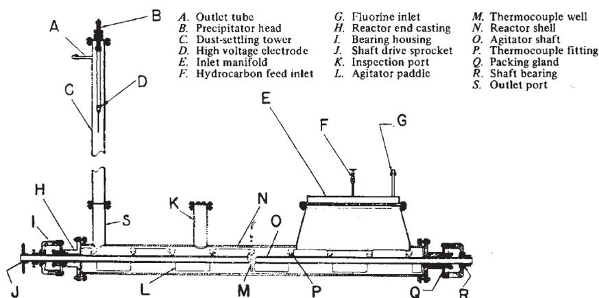
**Figure 2.2** Schematic representation of the apparatus used to perform the cobalt trifluoride process (courtesy of the American Chemical Society) [13].
