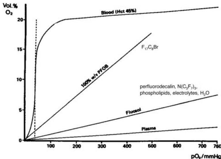
Figure 4.23 Oxygen-carrying capacity of human blood in comparison with pure perfluoro-*n*-octyl bromide (PFOB) and the blood substitute Fluosol [105] (graph modified from Ref. [102]).
